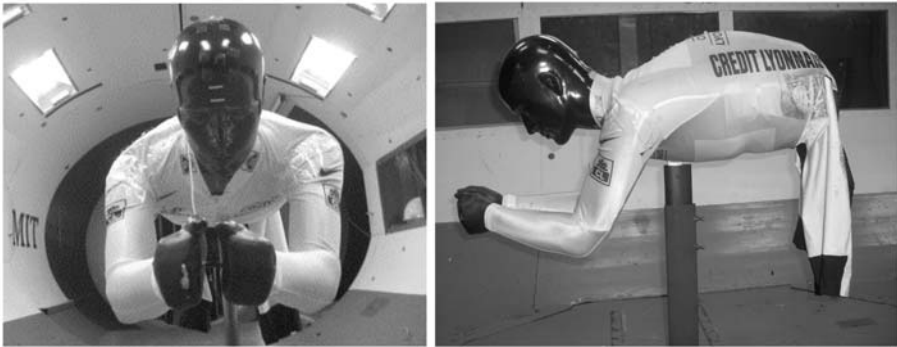
Figure 1 - Upper body mannequin in the wind tunnel. The lower half of the skin-suit was taped up behind the mannequin during testing.
